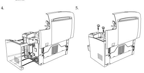
To confirm that the ROM module is installed correctly, print a status sheet. See "4 Testing and Connecting the Printer."
