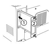
To confirm that the optional interface card is installed correctly, print a status sheet. See "4 Testing and Connecting the Printer."
